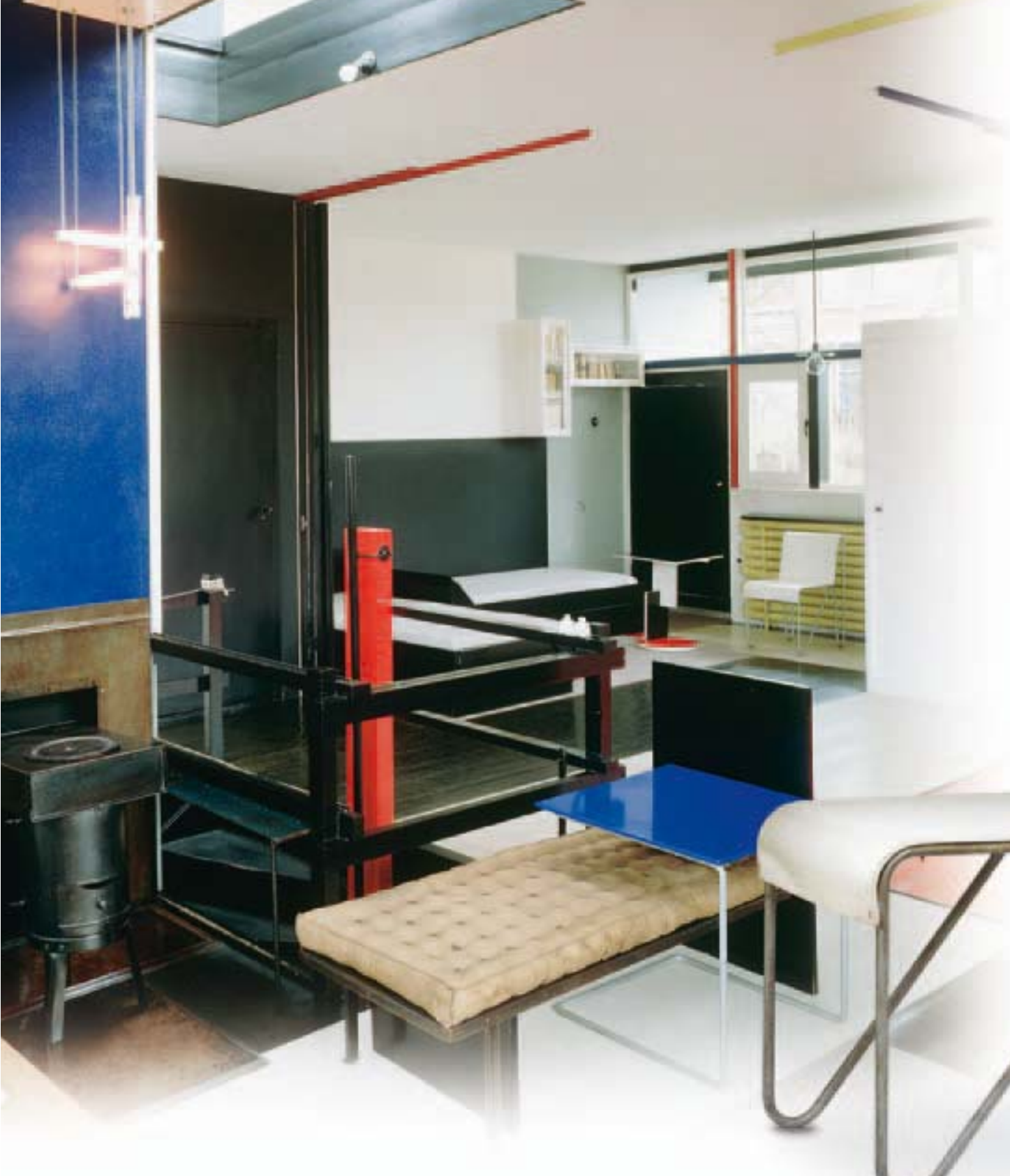
Interior of the Schroeder House, Utrecht, the Netherlands Built of steel, wood, and concrete, this early Modernist house is a composition of abstract planes. The moveable walls make it possible to transform the upper floor from a single space into a series of rooms. Furnishings and design by Gerrit Rietveld. 1924–25.
